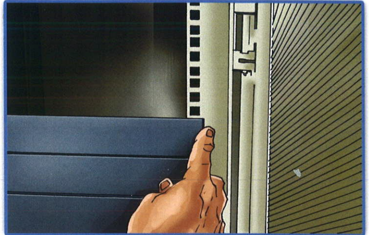
Place the panel in the required position and align the clips with the 19" mtg holes
