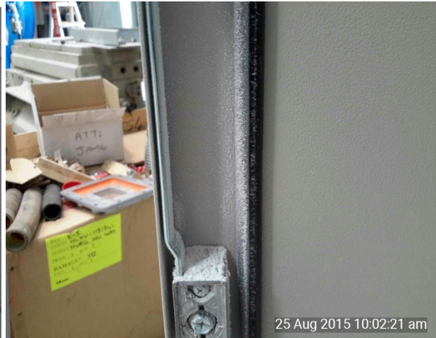
The enclosure before and after the IP6X test. No dust tracking into the enclosure was evident
