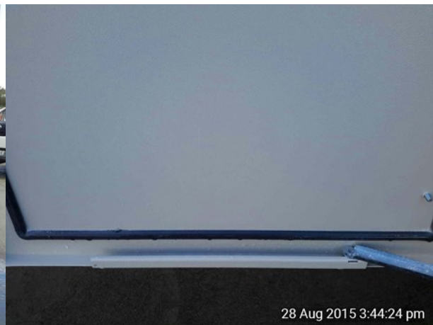
The enclosure before and after the IP6X test. No dust tracking into the enclosure was evident
