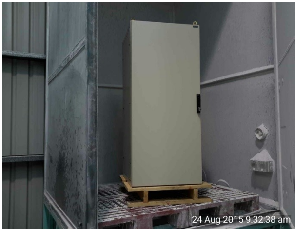
The enclosure before and after the IP6X test. No dust tracking into the enclosure was evident
